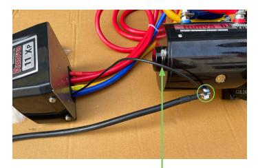
Detach the small black cable from the earth terminal on the winch motor.
